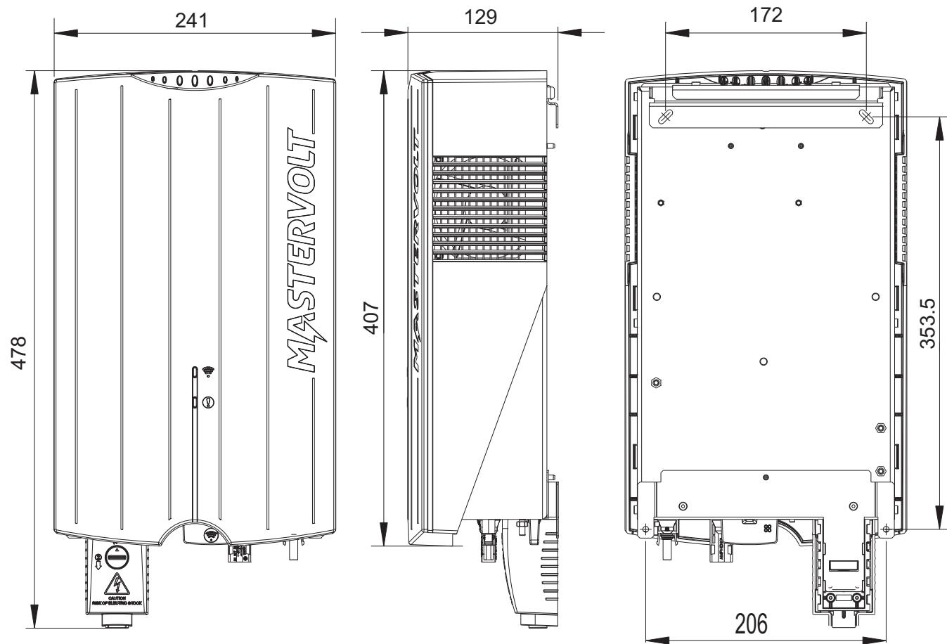
Figure 9-1: Dimensions of the Soladin 1000 Web and 1500 Web
