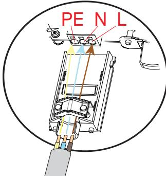
Figure 5-4: Connection of the AC cabling
